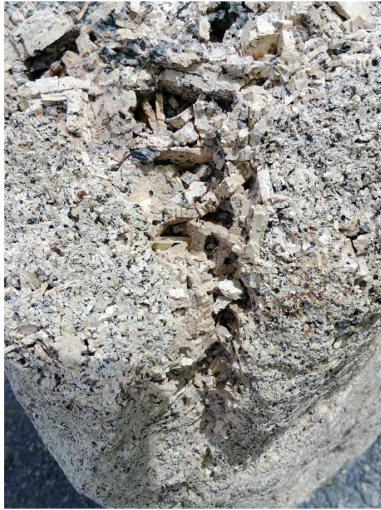
In situ vugs and cavities in the GMQ1 material
